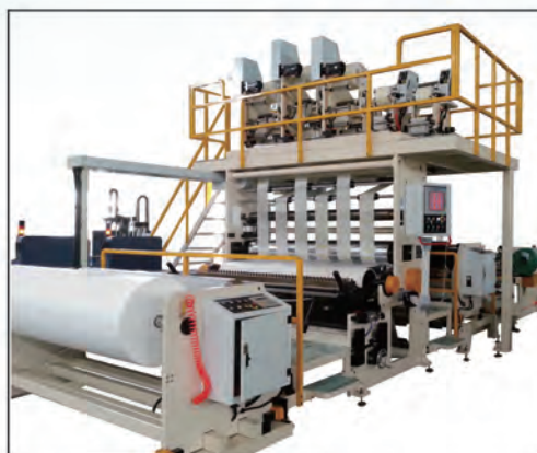
NT2400透气涂布复合设备 ▲ NT2400 Breathable Coating Lamination Machine
