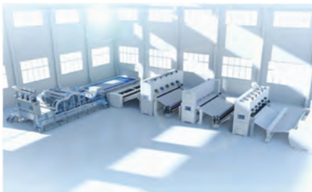
ANDRITZ high-capacity neXline needlepunch eXcelle for production of nonwoven technical felts
