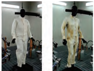
After Exposure Flash fire approx. 3 sec.
