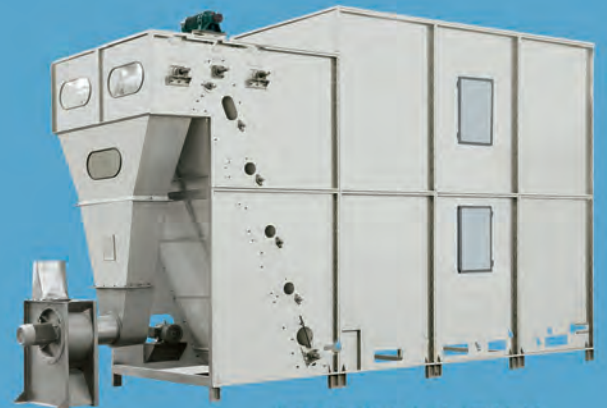
ASBG939大仓混棉箱 ASBG939 Large bin hopper
