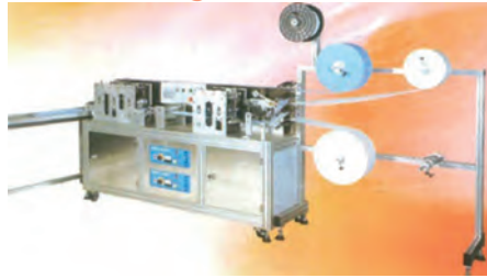
Mask blank making machine: 120pcs/min.
