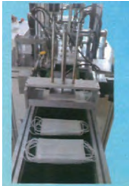
Ear looping sealing: 25pcs/min.
